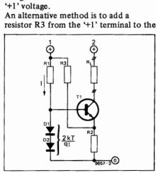
T1 emitter, as shown in figure 2. If D3 is chosen so that
